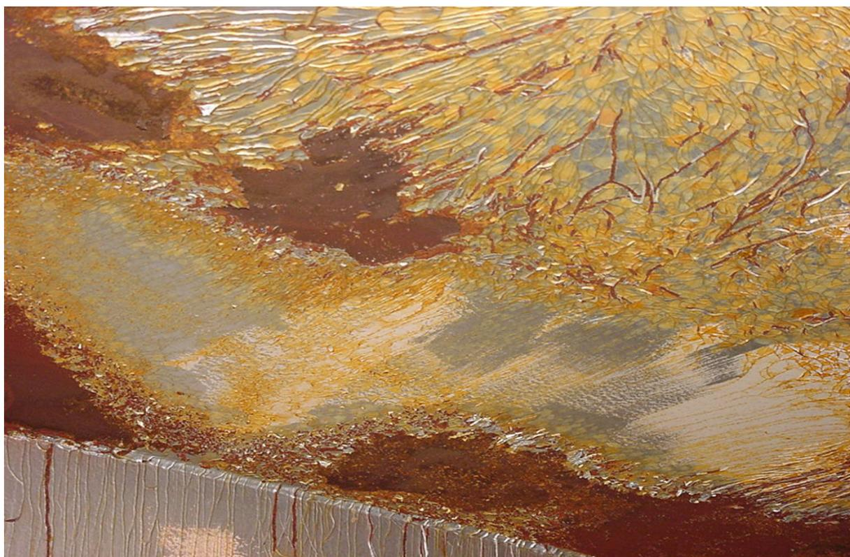
Figure 2. Catastrophic failure of a silicone high temperature coating.
